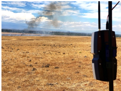
Fig. 1. Individual sensor node with multiple sensing modalities. Output from 3 different sensor modality during a fire event. The IR heat sensor shows an ignition with spreading. In addition, gas and particulate matter sensor reading show presence of obvious signatures of fire.
